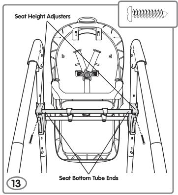
$\bullet$  From the back and bottom of the assembly, insert a #8 x 1,9 cm screw through both seat height adjusters and the ends of the seat bottom tube. Tighten the screws. This may require extra force.
